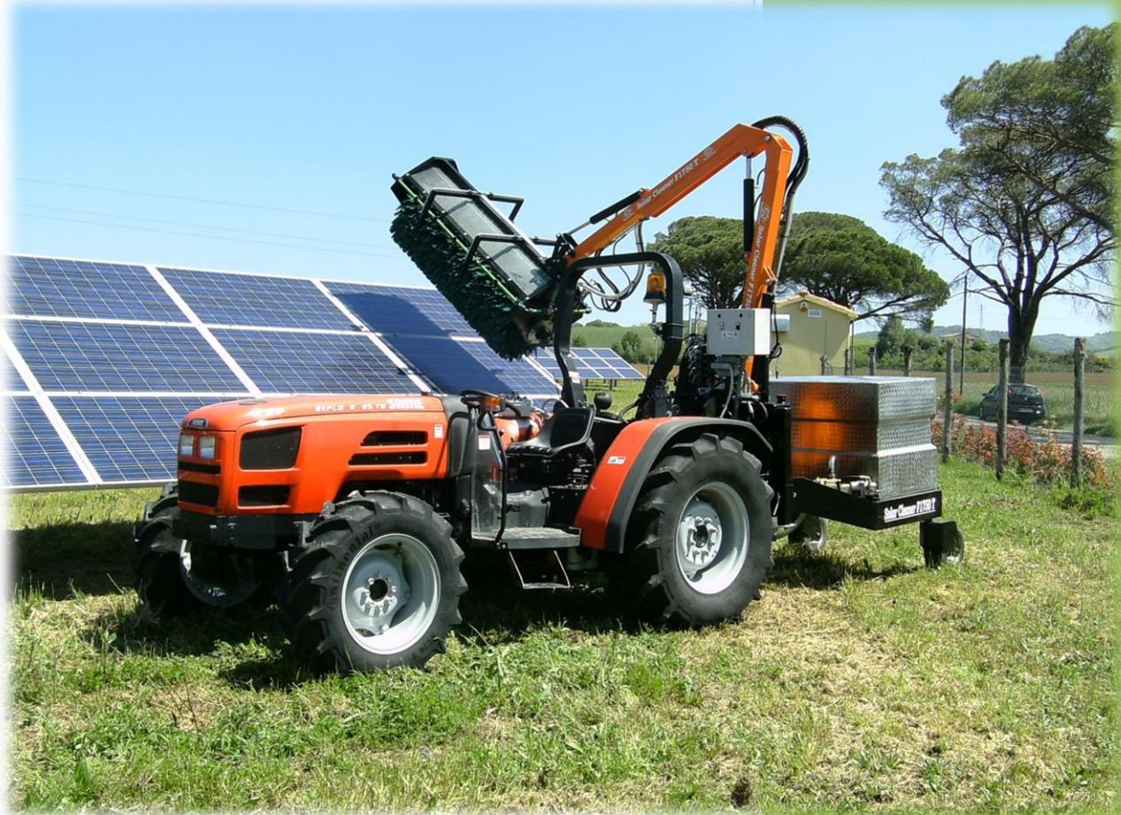
B.P. Metalmeccanica, focused on the needs of the PV industry's users, has expanded its range of machines for the panels cleaning on ground system, through the design and production of the new machine **SOLAR CLEANER F1750 T**.
